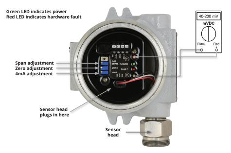
Figure 2: Sensor board components and zero/span adjustment
